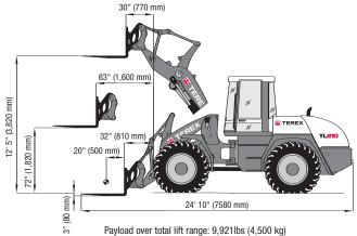
Payload over total lift range: 9,921lbs (4,500 kg) Payload in transport position: 11,023 lbs (5,000 kg)
