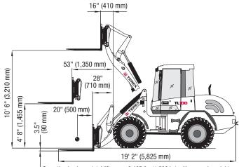
Operating load over total lift range: 3,497 lbs (1,586 kg) with rear axle weights Operating load in transport position: 4,410 lbs (2,000 kg) with rear axle weights
